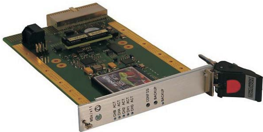
3U 4HP Controller board with CompactFlash site (Hard disk drive omitted for clarity)
